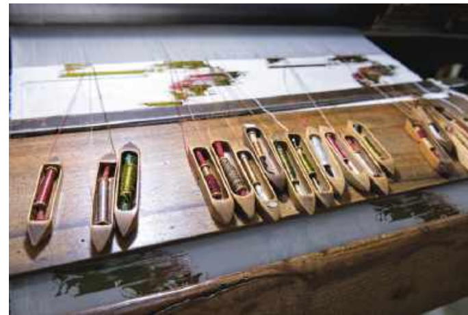
Demonstration of production of a brocaded silk fabric with dobby basis, 100% silk, in the 18 th century style on a 19 th century Jacquard loom; in the foreground, shuttles loaded with silk threads shoot between the warp threads.
